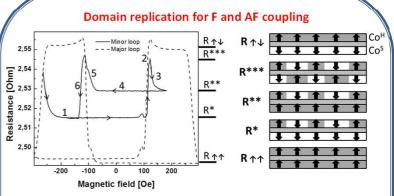
Major and minor magnetoresistive hysteresis loops. The minor loop is recorded for partially reversed CoH layer. The numbers 1-6 correspond to magnetic structure presented in bottom panel.
