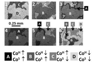
Domain structure recorded with P-MOKE microscope. The numbers 1-6 correspond to positions indicated on the R(H) dependence.
