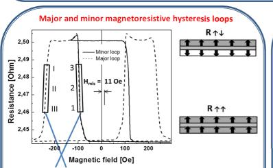
Major (dashed line) and minor (solid line) magnetoresistive hysteresis loops determined for Si/(Ti-2nm/Au-2nm)5/Au-2nm/Co-1.2nm/Au-2.5nm/Co-0.6nm/Au-2nm spin valve structure. H<sub>mls</sub> - magnetic field corresponding to the center of minor loop.
